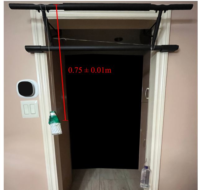
Figure 2. Two water bottles are tied to a pull-up bar to provide a counterweight system, allowing length adjustments of the string from the pivot point to the centre of mass, when need be.
